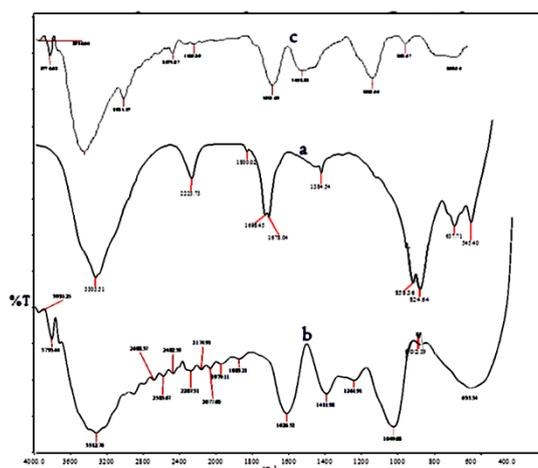
Fig. 2. FTIR Spectrum (a) Pure sodium molybdate (b) Pure *Aloe vera* (c) Film formed on metal surface after the immersion in well water containing 100 ppm SM - 25 ppm of  $\text{Zn}^{2+}$  and 10 ml *Aloe vera*
